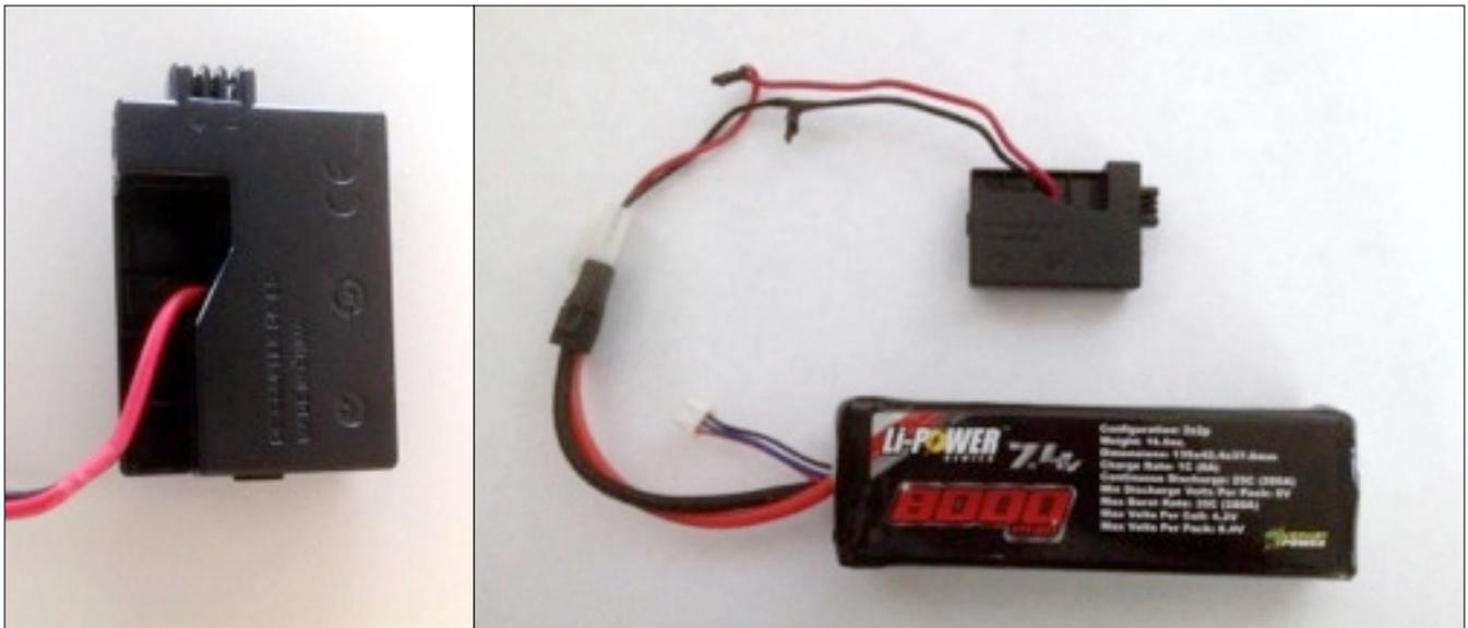
Fig 5. The assembled Coupler (left) and the battery-connector-coupler set-up (right)
