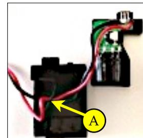
Fig 3. Drill hole location
